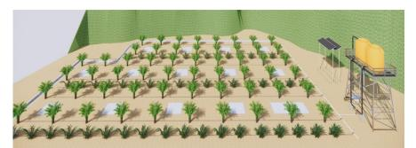
Figure 3. Lay-Out Schematic of Drip Irrigation System with Solar Energy.
