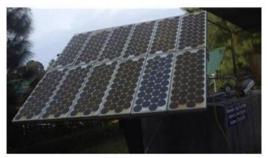
Figure 5. 28 Year Old PV Water Pumping System Showing Degradation at Hamirpur India (Chandel, Et Al., 2015).
