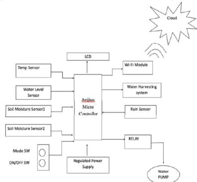
Figure 4. Block Diagram of Irrigation System Using Wireless Sensor Network (Pasha, et al., 2020)
